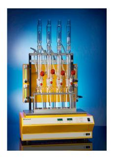
Digestion apparatus specifically developed for the decomposition and purging of water and soil samples for the determination of easily released cyanides and total cyanide, as well as other volatile gases.
